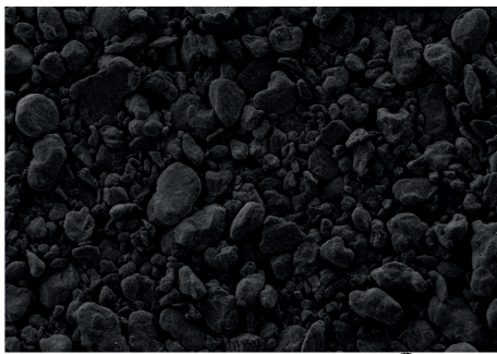
Tap density of rounded graphite 1,002g/L
