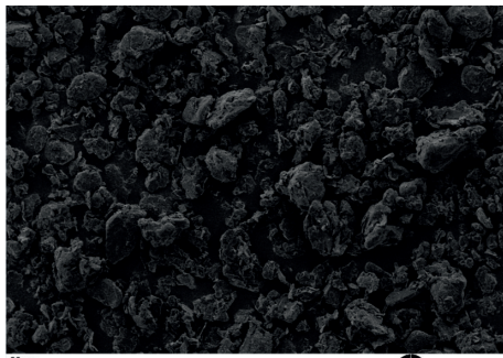
Tap density of feed material 691g/L
